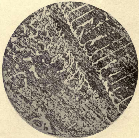
Fig. 18. \times 450 Alloy 20. Cu 66.2 Sn 4.2 Zn 29.6. Annealed at 450° C. \alpha + \gamma .
